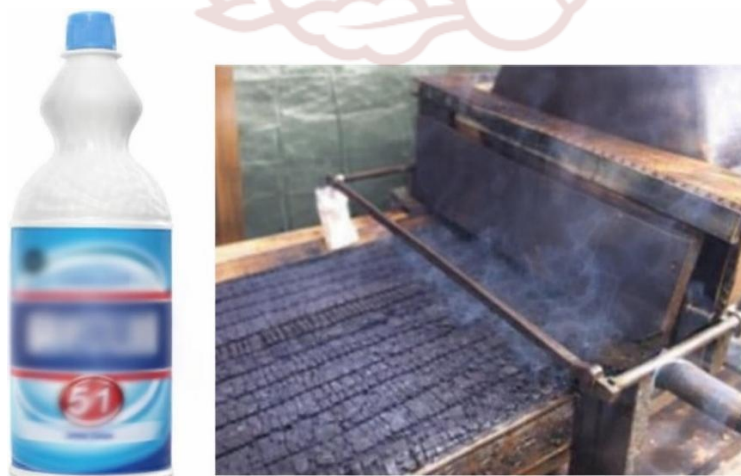
Figure 2. Carbonized Wood Surface after Controlled Burning
