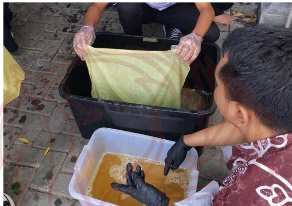
Gambar 19. Proses pencelupan zat warna sintesis Naphthol AS (Foto: Priyanto, Agustus 2023).
