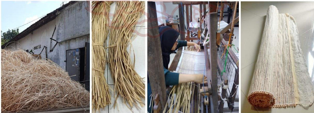
Figure 2: From left to right: (a) Waste from rattan splitting process; (b) Waste processed into rattan fiber strips; (c) Weaving process; (d) Roll of woven rattan fiber strip sheets, 1 meter wide.
