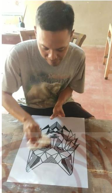
**Gambar 17.** Proses transfer gambar ke *screen* sablon
