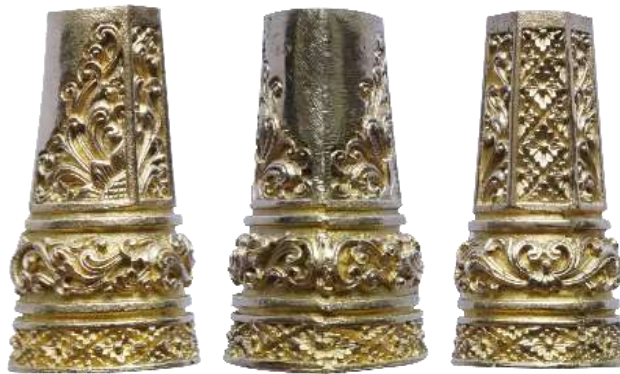
Gambar 207. Hasil pengecoran ( casting ) ali (Dokumentasi: Achmad Fathony, 2020)
