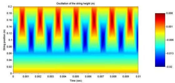
Figure 5. Vibration of a string with a bamboo clip that has a mass density 10<sup>6</sup> times higher than the string.
